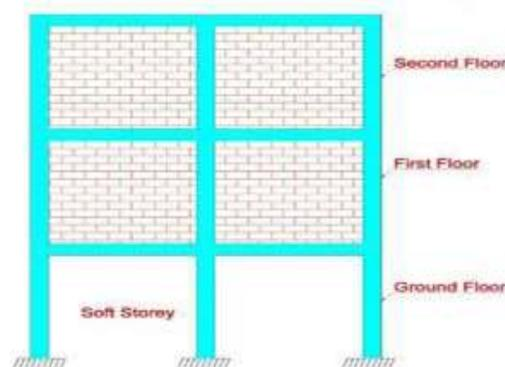
Figure 1.1: Soft storey structure
