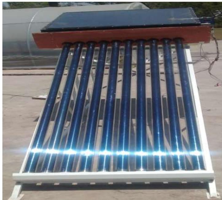
Fig. 1 Solar distillation system integrated with evacuated tube
