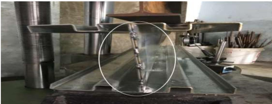
Fig 5 Lateral torsional buckling in web of cold formed I section with intermediate flange stiffener
