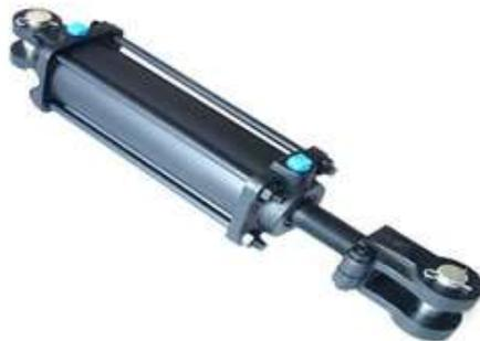
A hydraulic cylinder consists of a cylindrical barrel, piston, and a piston rod. The piston that is placed within the barrel is connected to the piston rod. The cylinder bottom, and the cylinder head, closes the bottom and the head of the barrel respectively. The cylinder head is the side from where the piston rod exits the cylinder.
