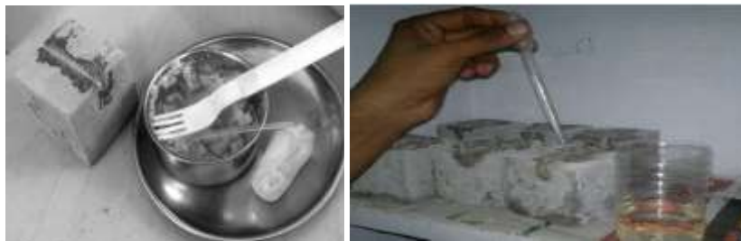
Fig. 1(a) Insertion of Bacterial paste into crack (b) Feeding Bacteria with Urathine-P
