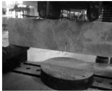
Figure -2 Flexural Test setup
