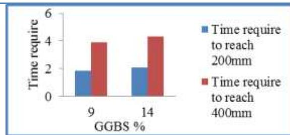
Fig. 7 L-box 200 mm & 400 mm time required
