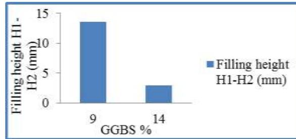
Fig. 5 U-box test results
