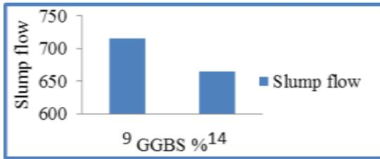
Fig. 1 Slump flow test Result
