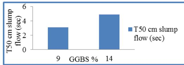
Fig. 2 Slump flow test T50 Result
