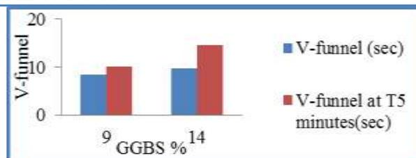
Fig. 4 V-funnel test results
