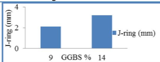
Fig. 3 J-ring test Result
