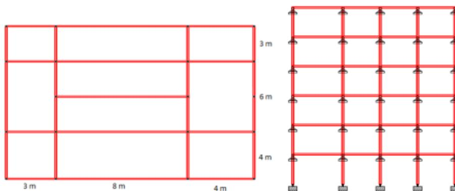
Fig : 1 : (a)Showing Staad building plan (b) side view of Staad model
