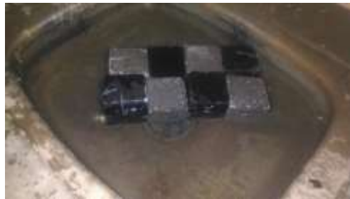
Fig-1 floating concrete
