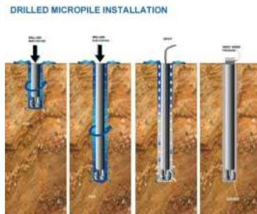
FIG1: Micro pile Installation[5]
