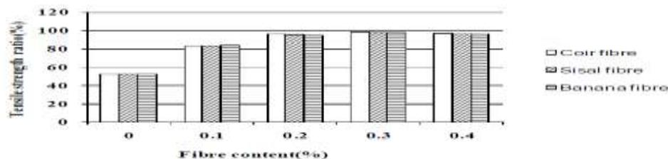
Hence, the final conclusion is coir fibre increases the tensile strength of bitumen and is also viable for use in commercial projects
