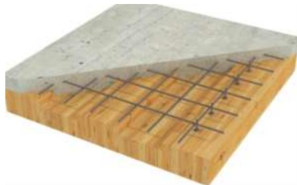
Fig. (c) Concrete with plywood (<https://images.google.com/>)
