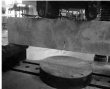
Figure -3 Flexural Test setup
