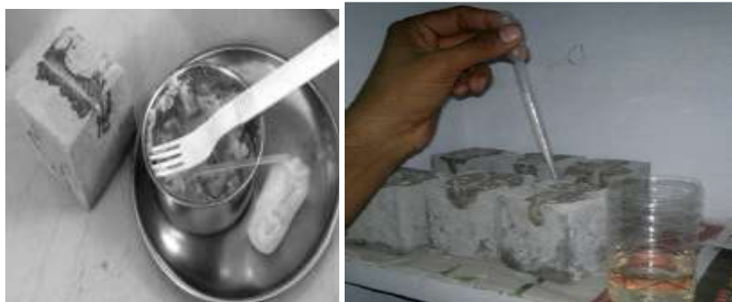
Fig. 1(a) Insertion of Bacterial paste into crack (b) Feeding Bacteria with Urathine-P
