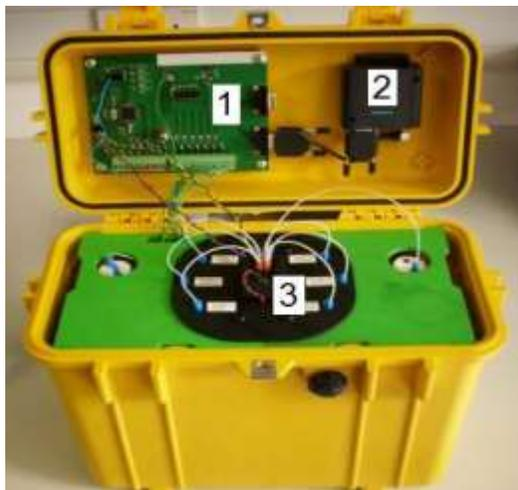
Fig-4. The prototype phosphate analyzer system. (1) Electronics board. (2) GSM modem. (3) Microfluidic chip / detector assembly. The battery, storage bottles, and solenoid pumps are contained within the lower part of the case.
