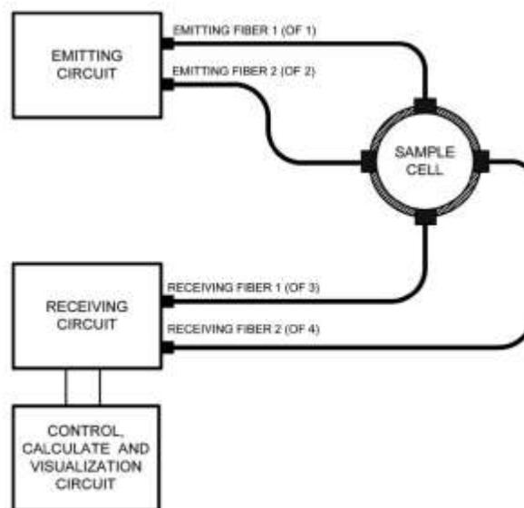
Fig-3. Basic block diagram of a four-beam turbidimeter.
