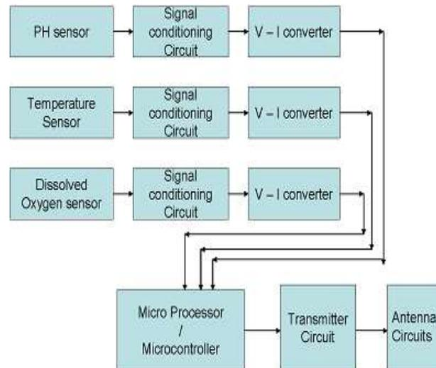
**Fig-8. Simple sensor node with different sensors mounted on it.**
