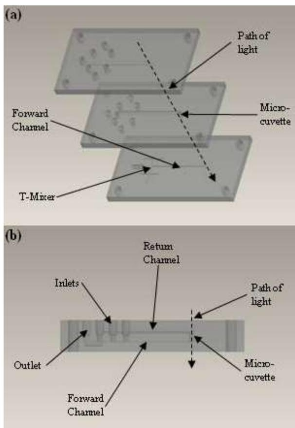
Fig-5. (a) Exploded view of the microfluidic chip. (b) Side view of fully assembled chip showing the micro-cuvette.
