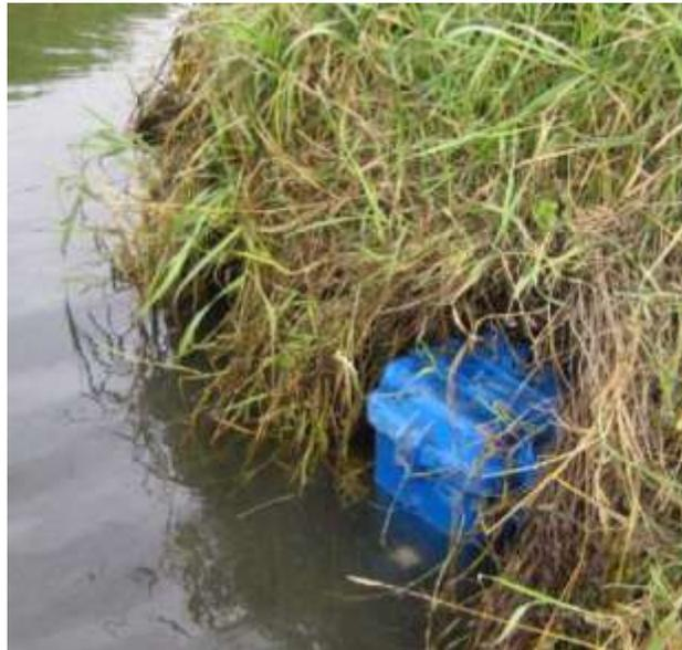
**Fig-6. The phosphate sensor in situ during the trial at Broad meadow Water, Co. Dublin, Ireland in September 2009. The sample inlet is visible below the water line.**
