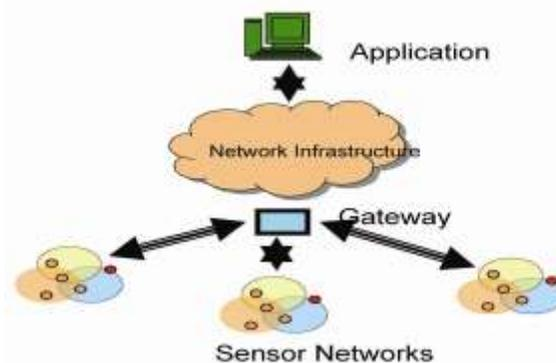
Fig-1. Wireless sensor network configuration
