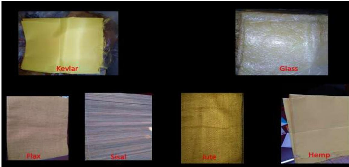
Fig: 2 Synthetic fibers (Glass & Kevlar) and Natural fibers (Jute, Flax, Sisal & Hemp)
