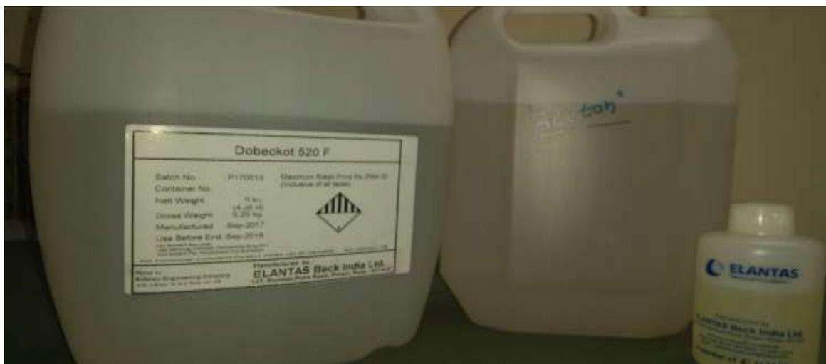
Fig 3: Polymer Resin (DOBECKOT-520F) and Hardener (ELANTAS- 758).
