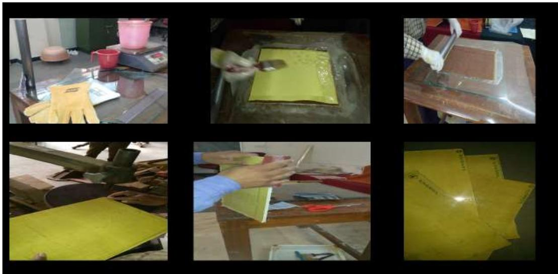
**Fig 4: Fabrication Set-up for Fiber Reinforced Composite**
