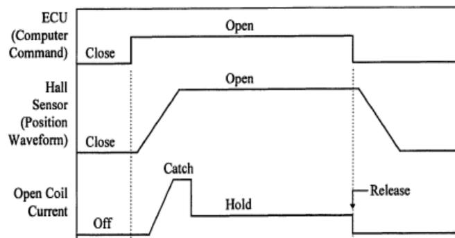
Figure 2: FEVAD Example Wave forms - Position and Current vs. Time
