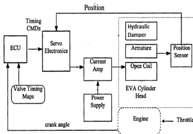
**Figure 1: FEVAD Electronics Configuration**
