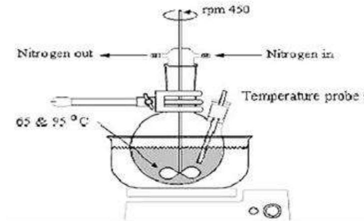
Reaction vessel for microsponge preparation by liquid-liquid suspension polymerization [12]
