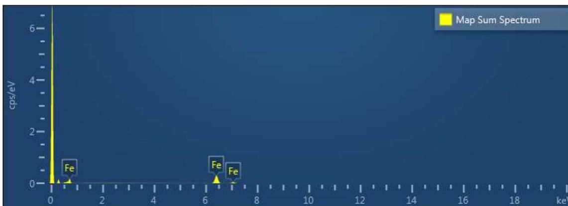
FIG: 2 EDS image of 250-300 mesh electrolytic iron powder.
