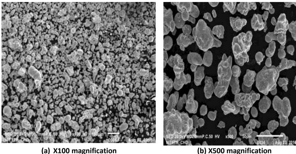
FIG: 1 SEM image of 250-300 mesh electrolytic iron powder.
