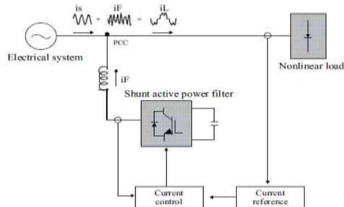
Fig 1. 2 Circuit Diagram of active Power Filter
