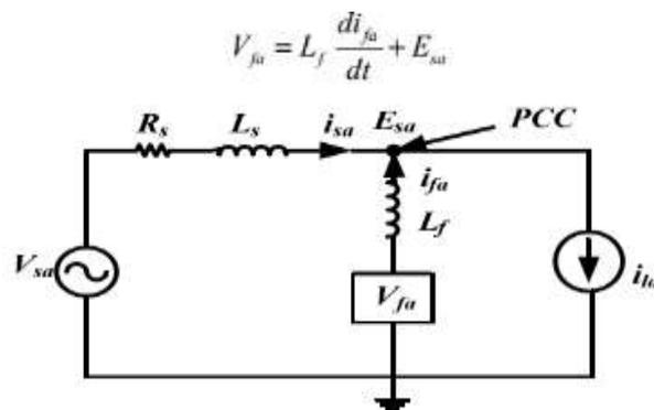
Fig 1.2 Single Phase equivalent circuit of APF
