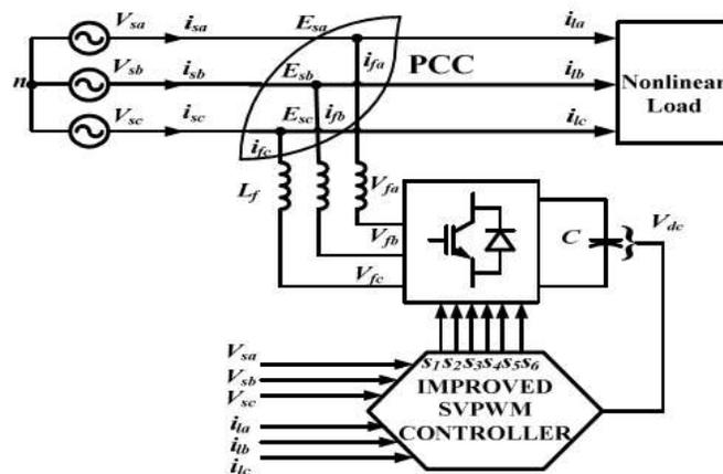
Fig 1.1 configuration of improved SVPWM based shunt APF
