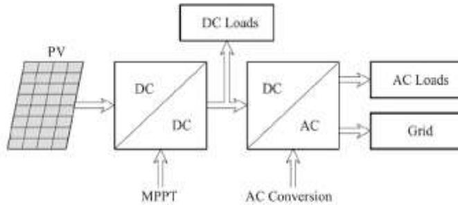
Fig.3. Block diagram of grid tied system
