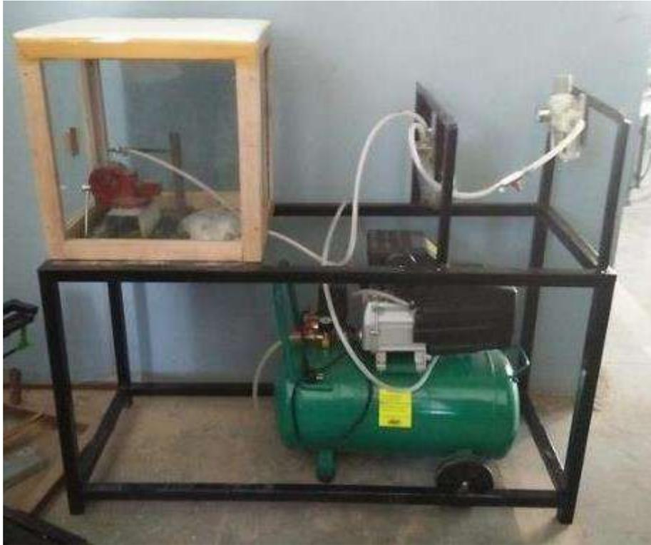
Figure 8: complete set up of abrasive jet machine
