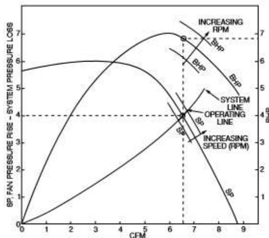
Figure 7. Variable Fan Characteristic Curve, Backward Inclined Centrifugal
