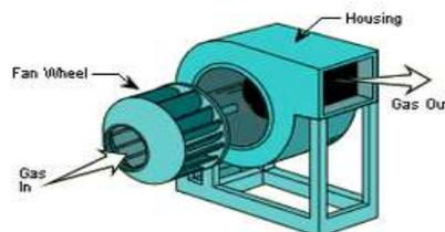
Figure 1: Components of a centrifugal fan
