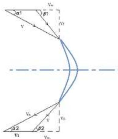
**Figure. 4 Velocity triangle for backward-facing blade**
