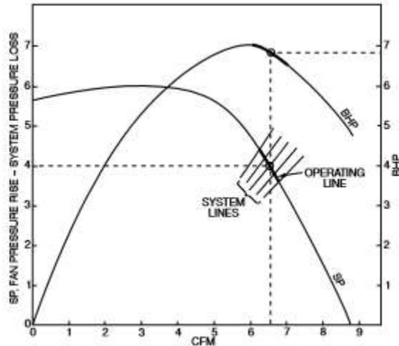
Figure 8. Variable System Characteristic Curve, Backward Inclined Centrifugal
