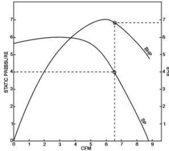
Figure.6 Static Pressure/Horsepower Curve Backward Inclined Centrifugal
