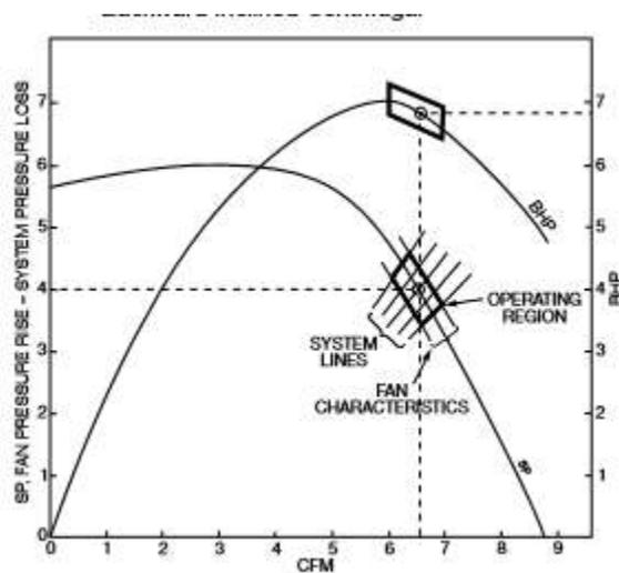
Figure 9. Variable Fan/System Characteristic Curve Backward Inclined Centrifugal
