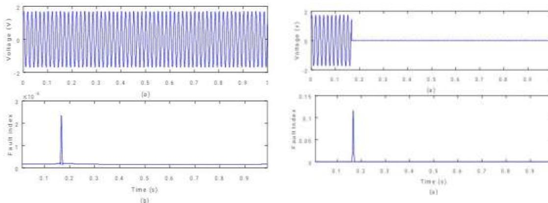
**Fig. 2. (a) Voltage signal (phase-A) (b) proposed median based fault index during LG fault.**
