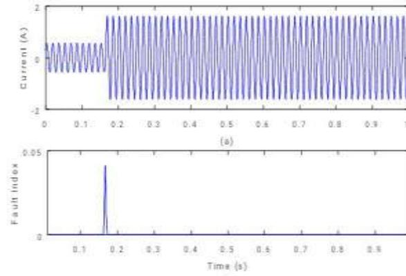
**Fig. 3. (a) Current signal (phase-A) (b) proposed median based fault index during LG fault. Double Line Fault**
