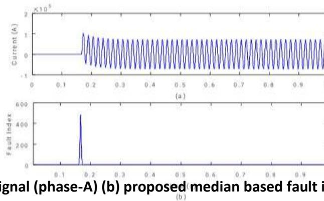
Fig. 7. (a) Current signal (phase-A) (b) proposed median based fault index during LLG fault.
