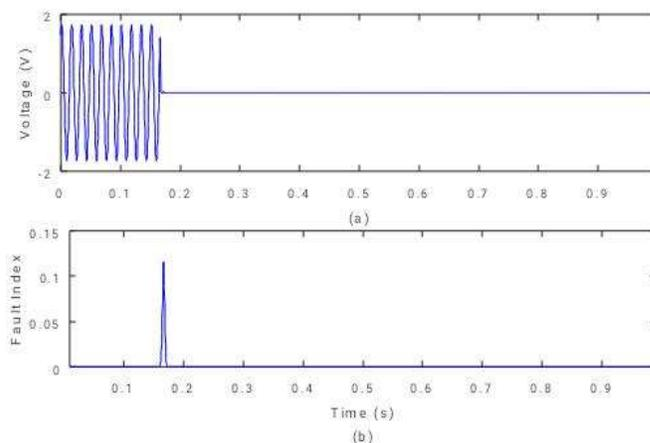
Fig. 6. (a) Voltage signal (phase-A) (b) proposed median based fault index during LLG fault.
