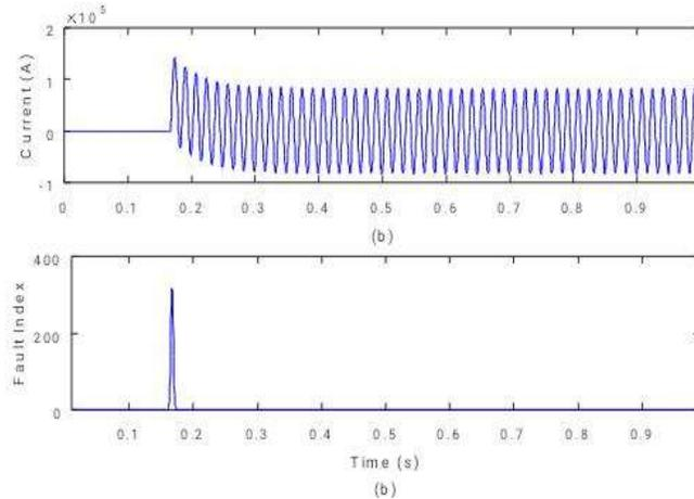
Fig. 9. (a) Current signal (phase-A) (b) proposed median based fault index during LLLG fault.
