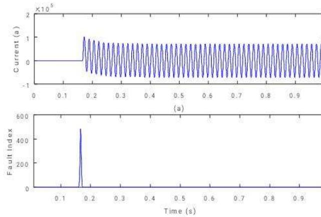
Fig. 5. (a) Current signal (phase-A) (b) proposed median based fault index during LL fault.
