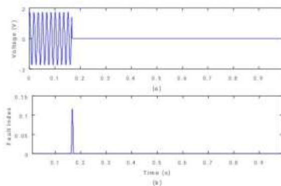
Fig. 8. (a) Voltage signal (phase-A) (b) proposed median based fault index during LLLG fault.
