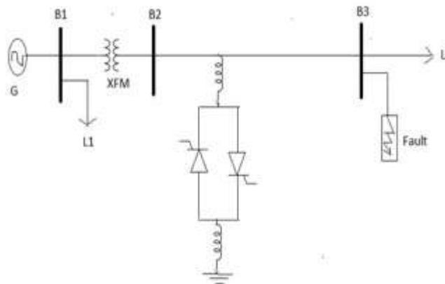
Fig. 1. Single line diagram of the proposed test system.
