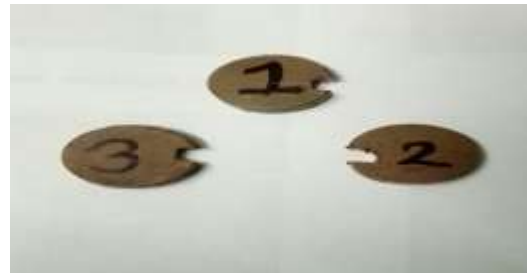
Fig 2. (a) Die (High speed steel) used for compaction (b) composites sample after the sintering 1) Cu-C 2) Cu - WC 3) Cu-SiC [Source: SGVU, Jaipur]
