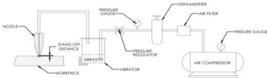
Figure 1: AJM Schematic Diagram [2, 3]
