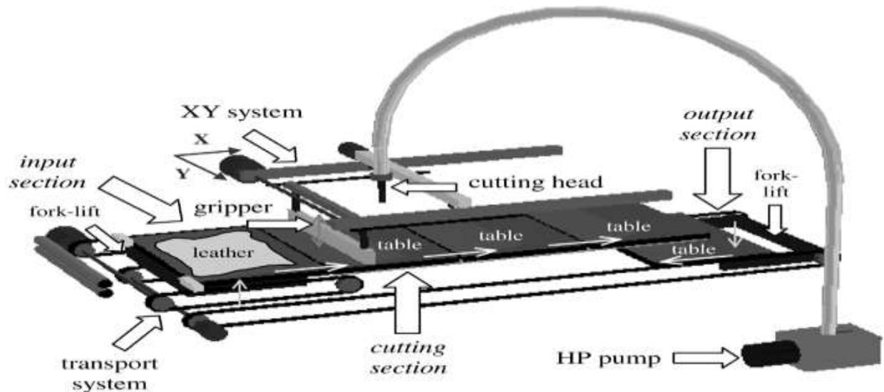
Figure 2: Schematic Diagram for WJM [5]
