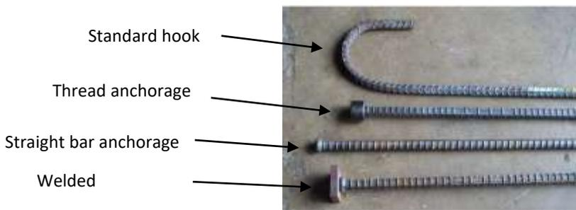
**Figure 1: Standard hook & Various mechanical anchorage (#8 size)**
