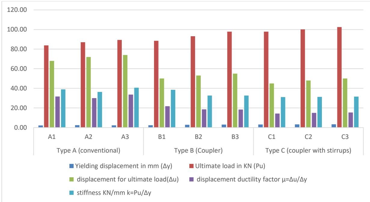
Figure 7 : Observed yield load, ultimate load ductility and Stiffness test
