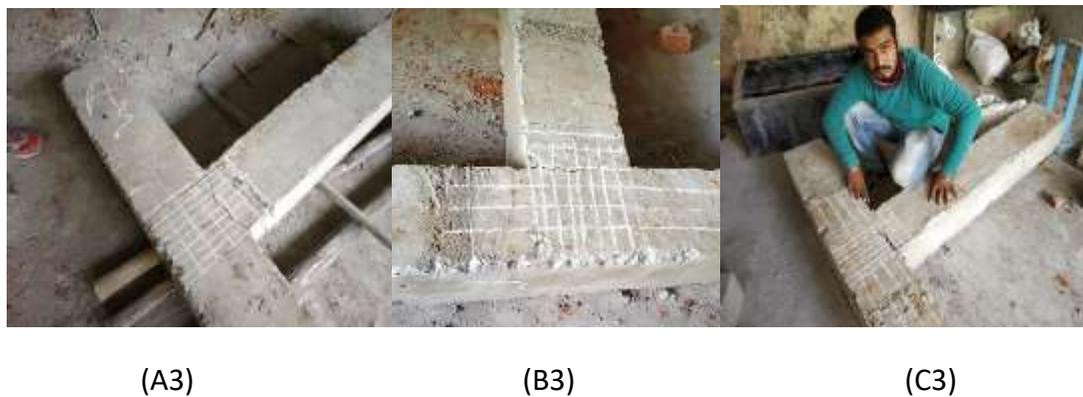
**Figure 11: Crack pattern of Group-3 (A3, B3, & C3)**
