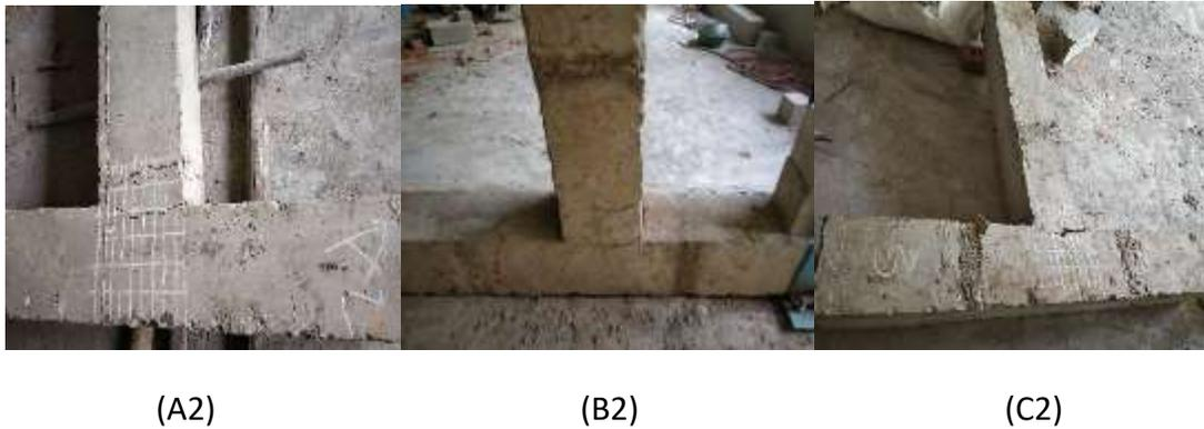
**Figure 10: Crack pattern of Group-2 (A2, B2, & C2)**
