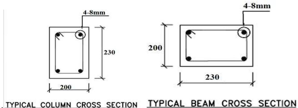
Figure 3 Beam and column size
