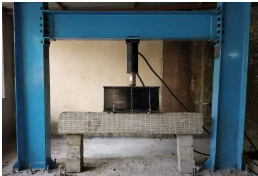
Figure 5: Filed arrangement of test setup
