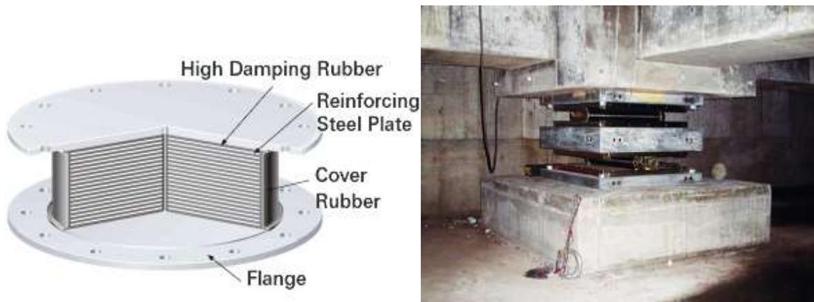
Figure 1:-Types of Isolators[<https://civildigital.com/base-isolation-system>]
