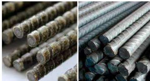
Fig: 2 basalt fiber bar & steel bar (Source: Google images)
