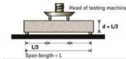
Fig:3 Two point loading test(Source: <https://civilblog.org/2015/06/24/flexural-strength-test-of-concrete-is516-1959>)
