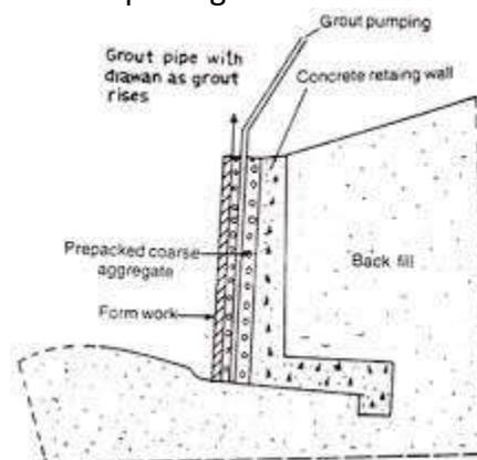
Figure 1 Pre-packed Aggregate concrete[1]
